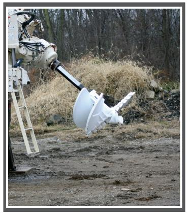
The Pengo PDD augers feature a cast heat treated head that provides superior wear and performance compared to normal fabricated augers. In addition the cast head is field repairable with standard welding techniques, utilizing low hydrogen welding rods and no pre or post heating requirement.
