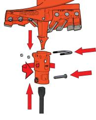
\*SAT-85 not recommended for anchor removal 1. Install SAT-85 over pilot bit of auger (Pengo FH-205 or FH-205C)
