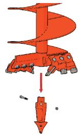
1. Remove pilot bit assembly from auger (1/2" hex bolt, 3/4" hex wrench)
