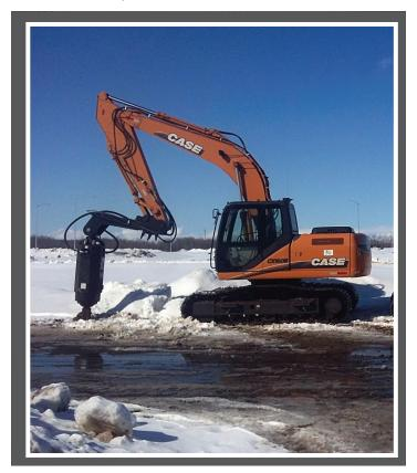
The RV-150 Series Variable Speed Drive is strictly for anchor installation due to it's ability to generate a high-level of sustained and consistent torque.
