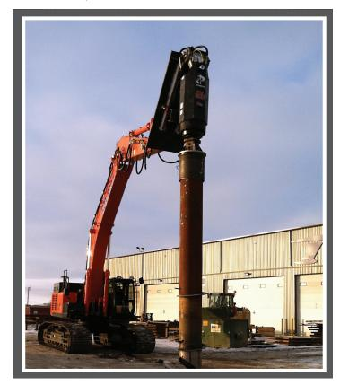
The RV-300 is the largest of anchor drives. It has the ability to power through the largest of anchor installation projects. Due to it's ability to generate a high-level of sustained and consistent torque it is not recommended for drilling.
