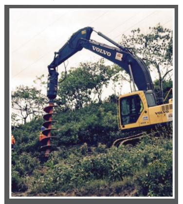
The RV-100 Series Variable Speed Drive is strictly for anchor installation due to it's ability to generate a high-level of sustained and consistent torque.
