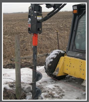
Pengo's Landscape Aggressor® is the perfect tool for landscaping applications or where smaller prime movers are required. Shorten flight bodies offers substantial weight reduction and performance is enhanced with our double entry flight design. Paired with our TriFlow® 350 pilot, providing three drill points for longer wear, the Landscape Aggressor® provides big performance in a small package.
