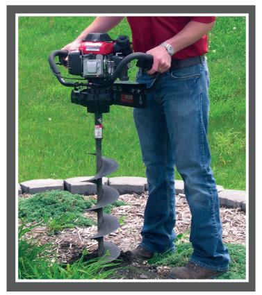
The Pengo's Hand Held Auger (HH Auger) is designed for one-man operation and is ideal for those light duty landscaping and fencing applications that require holes up to 8" in diameter and 36" in depth. Maintenance is made simple by the use of a one-piece head-treated cast head. Just insert, turn, and bolt.
