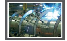
Reinforced support stanchions installed to reliably hold ribbon flighting.
