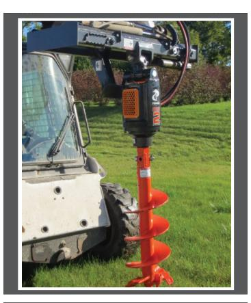
Pengo's latest addition to the Revolution Series Drilling drives are the CS Models. These models compact and light weight and are designed to work with our General Purpose 2" Hex Aggressor<sup>®</sup>, TriMax<sup>®</sup> and Severe Rock Ripper<sup>®</sup> augers. Combining this drive with the CS-2 Mount and your Pengo auger gives you a complete auger package.
