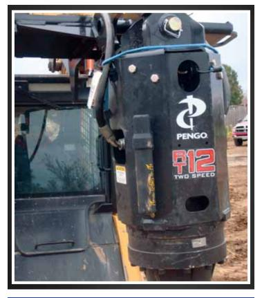
The RT-12 Anchor drive is perfect anchor installation projects when using a skid steer, mini-excavator or backhoe. This drive may also be used for some drilling applications with the Pengo Utility or Excavator auger system.
