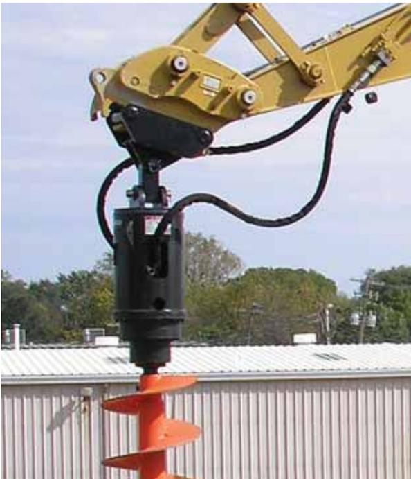
Pengo offers a complete mounting system for all sizes of excavators. These can be mounted directly to the boom or designed to work with an existing quick coupler. Excavator mounts allow for maximum movement to ensure the drive always hangs true to the ground. Pengo's mounts are available for the entire range of Revolution Series Drive Units.
