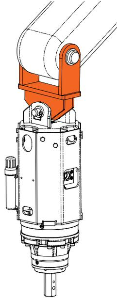
Pin the Mounting Bracket Directly to Boom of Prime Mover →
